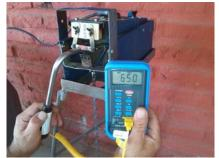
Pyrometer indicating proper blade temperature of 650°C.
